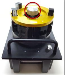
3.3.4. Open the Evo sample compartment and remove the front cover plate.
