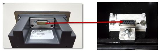
3.3.6. Ensure the CVC is fully seated on the sample chamber posts and that the front connector is engaged. See image below.
